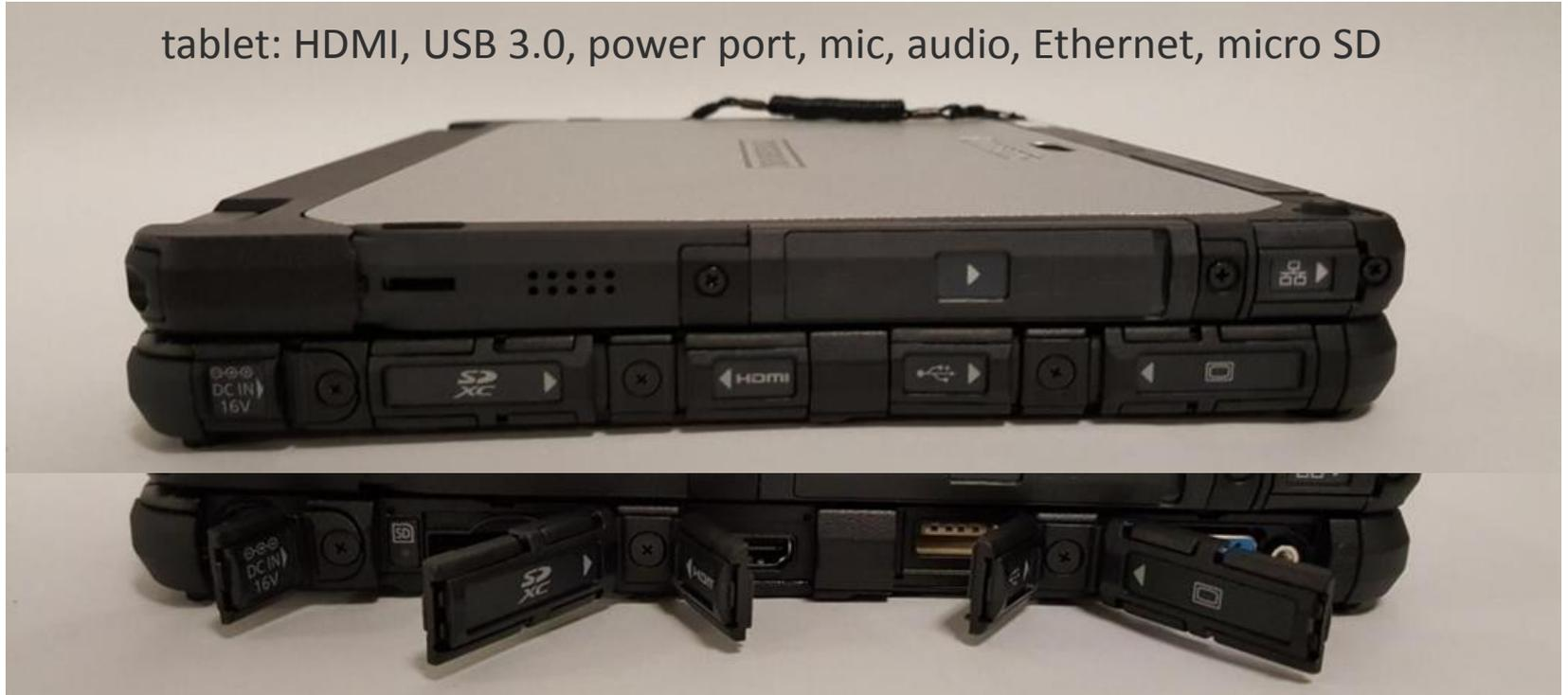
base/keyboard: power, SD card slot, HDMI, USB 2.0, VGA
