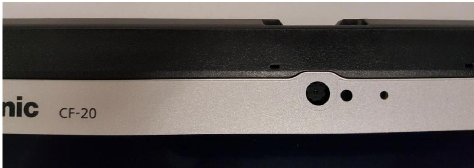
**Docking the tablet:** insert it straight down and push until the orange rectangle disappears. If not fully docked, you'll carry it by handle and tablet can fall out. Also get in habit of locking the front latch.
